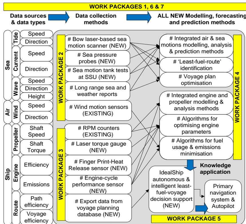
Figure 4. AutoSet System and data flow diagram
