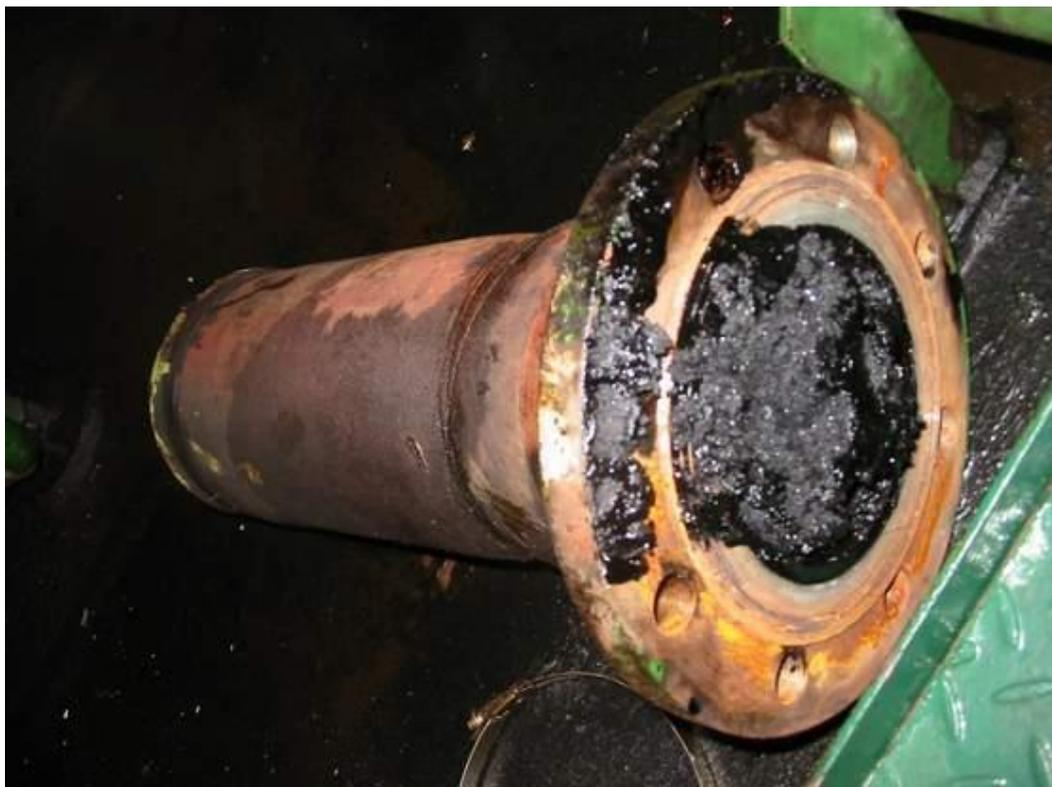
**Figure 11.4.1 - Clogged fuel pipes due to very poor quality fuels**
