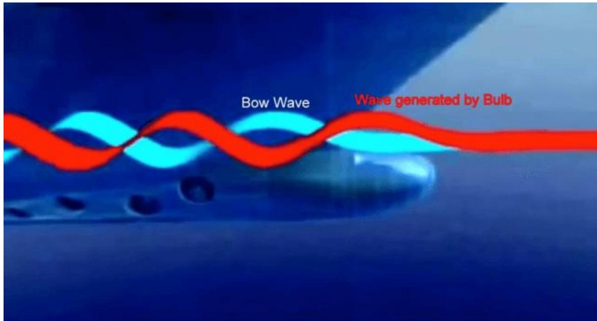
**Figure 12.4.1 – Concept of bow waves and bulb waves that cancel each other**
