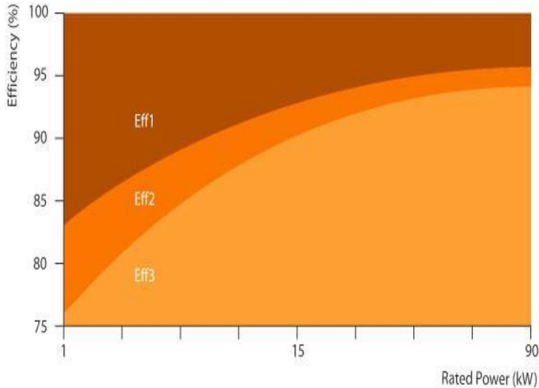
**Figure 12.6.1 – Example of energy efficiency rating of electric motors**
