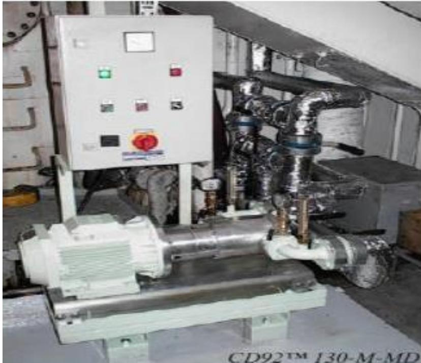
**Figure 12.6.2 – Typical homogeniser**
