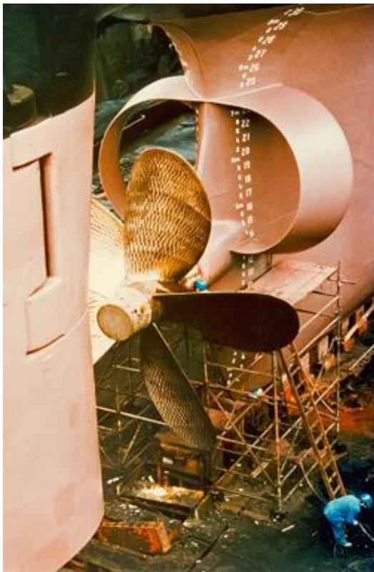
**Figure 12.1.2 – Typical wake equalising duct [Scheneekluth]**
