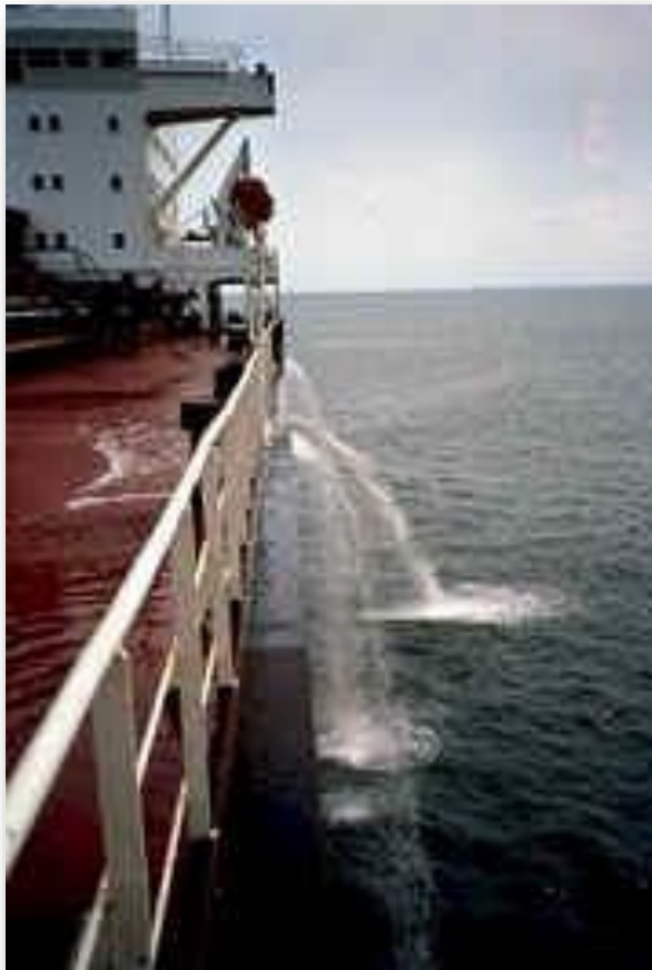
Figure 4.5: Ballast water exchange using flow-through method
